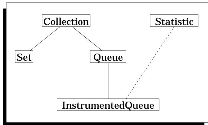
The solid lines indicate which classes are subclasses of others. The dashed line indicates that `InstrumentedQueue` has local fields of class `Statistic`.
