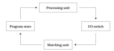
If no match for the arriving token is found in the matching store, the token is written into storage and held in abeyance for matching tokens expected to arrive in the future. For unary operators, no matching is needed, and the token can bypass the matching unit and proceed directly to the program store. It is estimated that 55–70 percent of all tokens are able to bypass the matching section.
